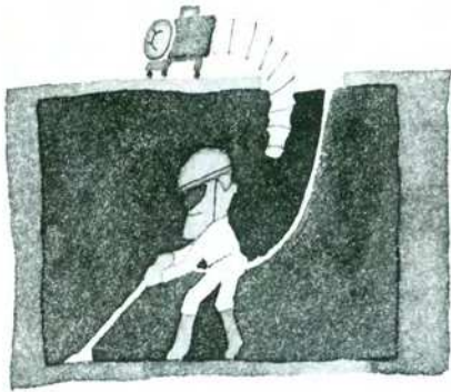
Sump pit ventilation
